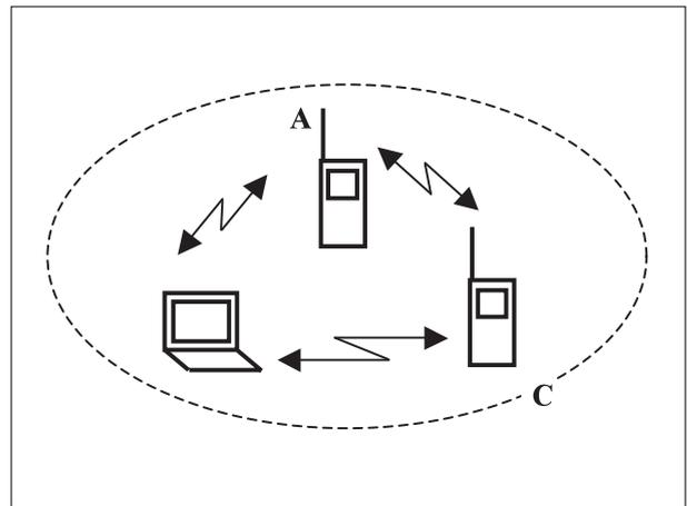
\* terminal is autonomously connected to others and can communicate each other without passing the cell station.
