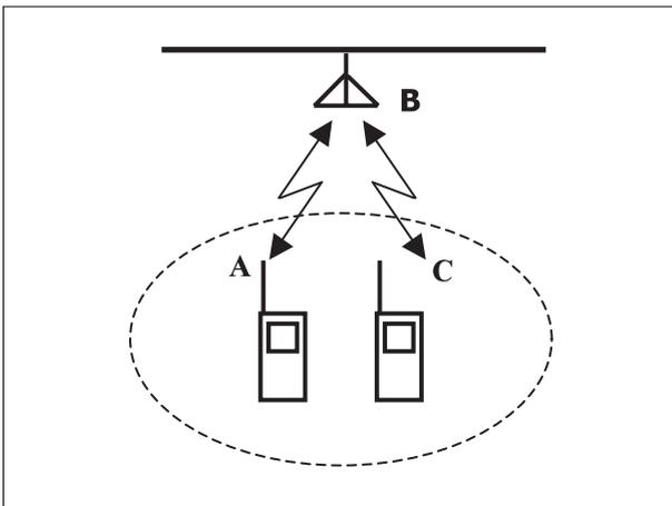
\* Even if user A and user C are in the same mobile cell, communications between them have to pass the cell station B
