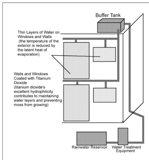
**(1) Cooling of surface temperatures through engineered evaporation systems**
